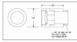
The Model 1153 converts a Model 211 illuminance sensor to a Model 2153 Brightness Sensor. It is intended for users who wish to make both illuminance and luminance measurements with a single sensor.
