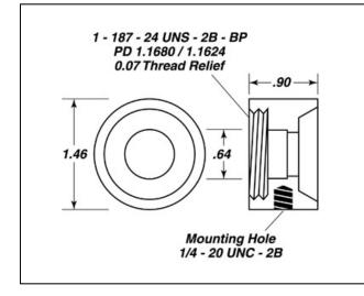
This Universal Sensor Housing holds a standard 1 cm<sup>2</sup> BNC detector package and is a component of UDTi Standard Series sensors. Includes a male-threaded adaptor (Model 108) which connects directly to Standard Series filter holder (Model 104) attenuators and integrating spheres.
