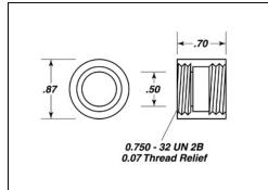
Designed to hold 12.5 mm diameter filters the Model 104-MINI connects male-threaded Miniature Series sensors and accessories.
