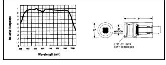
The Model 247 is UDTi's Miniature Series flat response radiometric sensor. It can be adapted for use with Miniature Series accessories.
