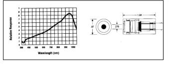
The Model 264 is a Miniature Series sensor specifically designed for laser power measurement. It consists of a Model 260 type sensor with a built-in diffuser and reduced aperture for attenuation of optical power.
