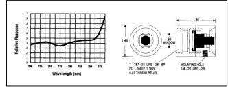
The Model 222 is a Standard Series silicon sensor calibrated in the UV region (200 - 400 nm)
