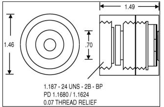
The Model 2550 uses separate layers of diffuse material to attenuate radiation reaching a sensor thereby increasing input power capacity. It is compatible with Standard Series sensors.
