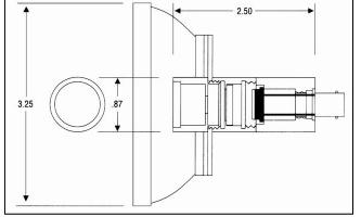
The model 2153 is the UDTi standard luminance head with an integral lens that provides a fixed field-of-view of 13 degrees. It is suitable for measurement of the brightness (luminance) of diffuse surfaces or uniform light sources.
