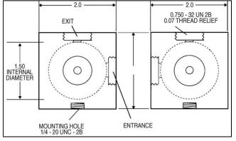
This 50 mm diameter integrating sphere features a 10 mm entrance aperture. This sphere is suitable for testing of larger fiber/beam diameters. Compatible with Miniature Series sensors.
