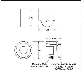
This accessory holds our standard 1cm<sup>2</sup> silicon photosensors. It is provided with five interchangeable apertures.
