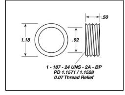
The Model 108 coupler is designed to connect two female-threaded Standard Series accessories.
