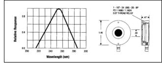
The Model 268UVC is a Low-Profile Series radiometric sensor optimized for measurements in the UVC region (200 - 280 nm).
