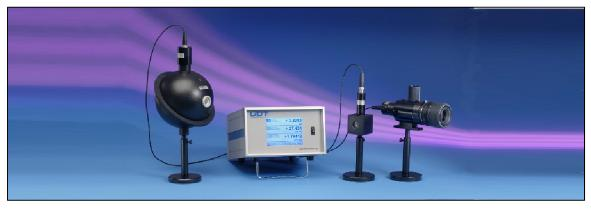
An *optometer* measures the photocurrent produced by a photometric or radiometric sensor, applies a predefined electro-optical calibration factor, and displays the result in optical units. A *photometer* system is built by coupling an optometer to a photometric sensor; a *radiometer* system is built by coupling an optometer to a radiometric sensor.
