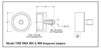
1700-Series Fiber-Optic Adaptors are compatible with UDT Instruments Miniature Series Sensors (Model 260, 261 and 280). Details are provided in the following brochure:
