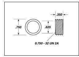
The Model 108-MINI coupler is designed to connect two female-threaded Miniature Series accessories
