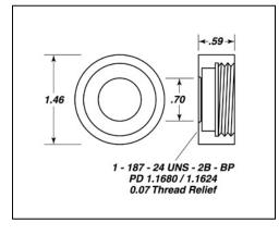
The model 102 Filter Holder holds any 25 mm diameter filter. It is femalethreaded on one side for connection to Standard Series sensors.
