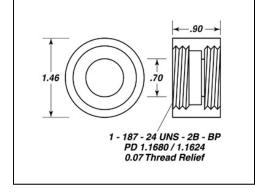
Designed to hold standard 25 mm diameter filters the Model 104 connects male-threaded Standard Series sensors and accessories. While the Model 102 Filter Holder is threaded on one side only both sides of the Model 104 are threaded to permit stacking of accessories.
