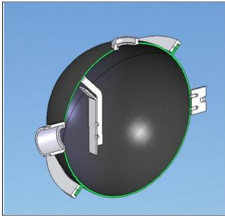
Sectional View - Model 2500 or 2525 - Note that the design of the two models differs only in the size of the aperture mounted at the sphere's sensor port.
