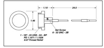
For luminance measurements in difficult to reach places such as in photocopiers or photolithography systems UDT Instruments offers two luminance probes. Both are fiberoptic bundles. The model 116 is two feet long 0.25" fiber core which couple to the Model 211 sensor head. Standard Calibration(s) nit (cd/m<sup>2</sup>); footlamberts Aperture diameter (mm) 6.35 Dynamic Range 1.0E-02 - 1.0E+05 cd/m<sup>2</sup> Compatible Components 211
