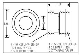
UDT Instruments' bandpass filters provide a 10 nm half-power bandpass (FWHM) at peak wavelengths corresponding to common laser lines. Assembly includes a Model 104 Filter Holder. Other types of bandpass filters are available as special order items.
