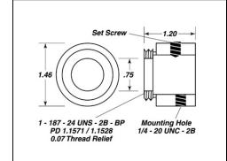
The Model 1718 is designed to couple female-threaded Miniature Series sensors and accessories to male-threaded Standard Series accessories.
