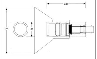
This luminance head was specifically designed for measuring display brightness. Its integral lens provides a fixed field-ofview of 13 degrees and a miniature fixed rubber light shade eliminates errors due to ambient light and keeps the display from being scratched during measurement.
