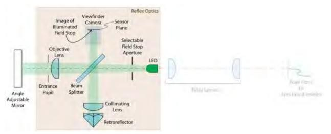
Figure 4. Schematic of the optical layout of the Gamma Scientific NED Measurement System in "viewing mode," and with an adjustable mirror in front of the NED. Aligning the optics to this mirror enables the system to take measurements from both the left and right side of the NED without any change in pointing direction.
