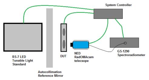
Figure 2. Schematic of the main elements of a system for performing high precision measurements of absolute color and luminance on NEDs. Mechanics for controlling the position and pointing direction of the telescope are not shown.
